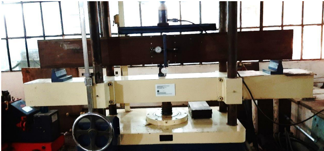
Compression Testing Machine for Beam
